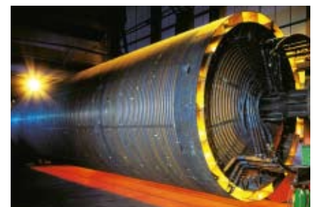
Using heat optimally: The heat recovery boiler's pipelines heat both liquid and gaseous media to high temperatures.
