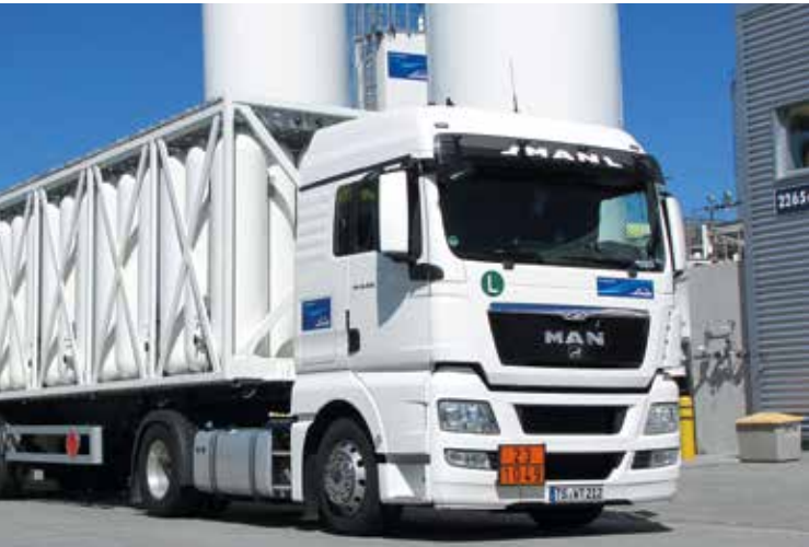
From the plant to the pump: The new 500-bar storage technology allows a trailer (above) to transport twice as much hydrogen. This reduces delivery trips and benefits hydrogen refuelling stations like here in Berlin, Sachsendamm (left).
