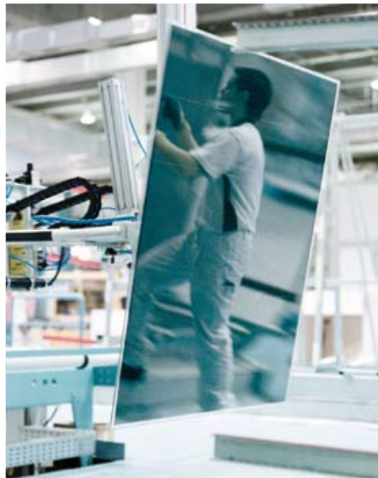
High tech for solar electricity: in Spain's first factory for thin-film solar cells, 2.2 x 2.6-metre large solar modules are manufactured from nitrogen, hydrogen and climate-neutral fluorine.
