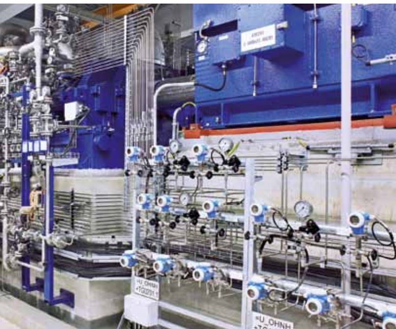
Pre-injection stage: The oxyfuel pilot plant with integrated flue gas scrubbing at the Schwarze Pumpe power plant supplies high-purity CO 2 .
