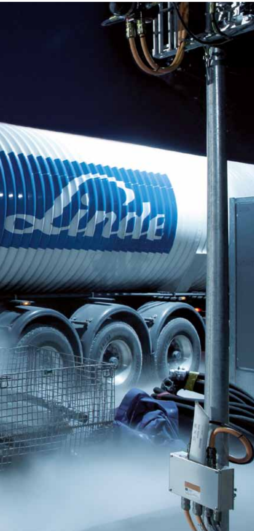
Temperature extremes: The liquid nitrogen in the tankers is maintained at minus 196 degrees Celsius (left). Damp air condenses to form frost on the ice-cold pipes in August 2011 (bottom). Following delivery (top), the cryogenic cargo is vaporised for the inerting step. Heat exchangers warm the N 2 up to 40 degrees Celsius.
