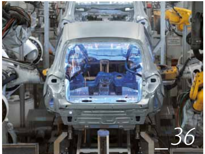
WELDING TECHNOLOGY: Shock freezing helps to "relax" hot welds
